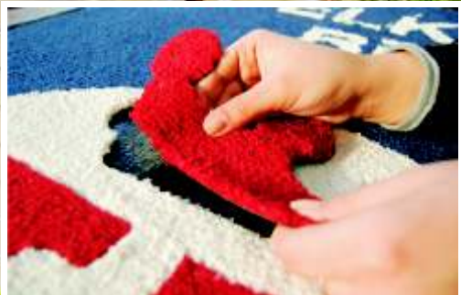
Graphic-Inlay® mats are precisely machine cut then hand assembled by skilled craftspeople.
